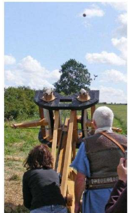
Postscript Plate 2. (left) In 2009 Len Morgan completed this very impressive full-size reconstruction of a Vitruvian ballista for a 2 librae (0.655kg) stone shot, the smallest ballista on Vitruvius' list. It is based on my revision of Vitruvius' Latin text and the model in Plate J. The improved Mk II version is likely to be ready in August 2011. (right) Appropriately, one of the first test shots was aimed and released by Dr Pam Rose, without whose enthusiastic cooperation this survey of artillery missiles would never have been written.
